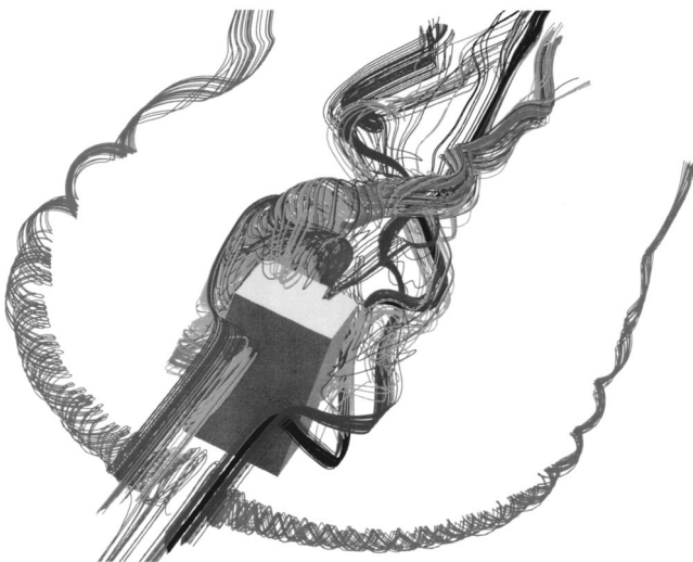
FIG. 14. Three-dimensional flow evolution pattern revealing the process of vorticity cancellation and local disappearance of the wake at t=14 , Re=500 .
